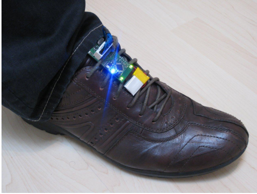
Figure 5. The Planipes sensor board is attached on the instep of the test person’s shoe.
