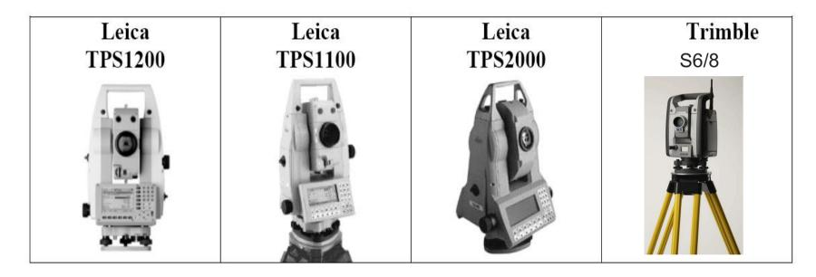
not yet specialised for that purpose (still can be used manually) problems: sensitive electronic, optical sight (fog), price, need for prisms
