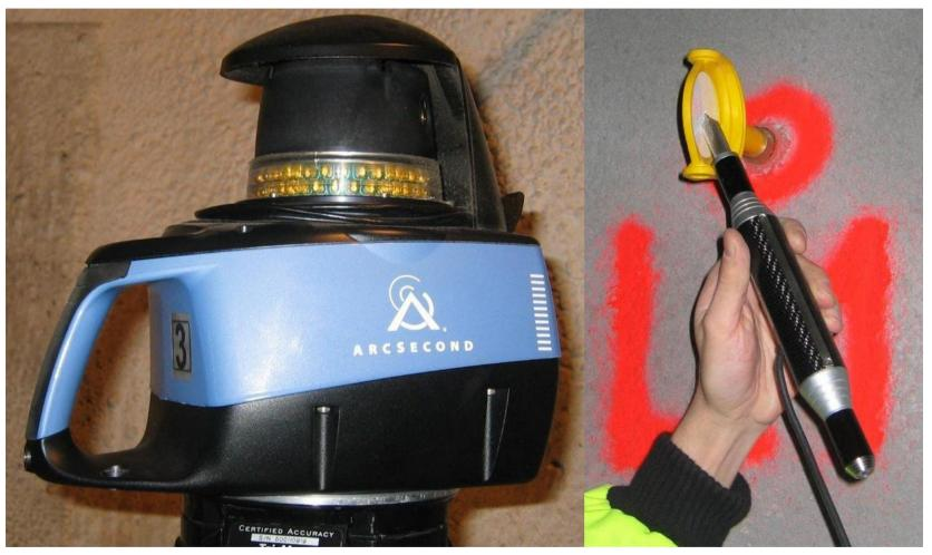
iGPS transmitter and sensor during a test in a tunnel
