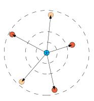
Every node i measures its distance  $d^i_j$  to all other nodes j in the same ring and calculates the coordinate tuple  $\langle d^i_1, d^i_2, \ldots, d^i_{k+l} \rangle$  where  $d^i_i = 0$ .
