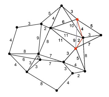
LocaLISE constructs a minimum-interference t-spanner
