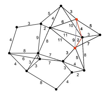
LocaLISE constructs a minimum-interference t-spanner
