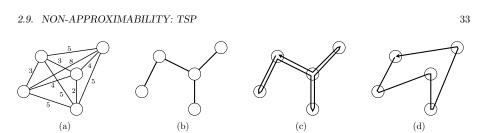
Figure 2.67: A weighted complete graph as an input to TSP (a), an MST in this graph (b), the tour  $P_0$  obtained from this MST, starting from an arbitrary node (c), and the simplified tour P after removing repeated occurrences (d).
