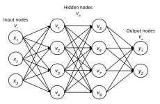
Figure 6.4: Example of a neural network for an input  $\boldsymbol{x}$  and an output  $\boldsymbol{y}$  with three input nodes, eight hidden nodes and two output nodes.
