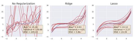
Figure 5.25: Fitting a polynomial of high degree to a cubic function with and without regularization. We see that variance and total error drops when regularization is added.
