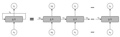
Figure 6.24: Unrolling the RNN through time. At each time step,  $\hat{g}$  and  $\hat{h}$  compute output  $y_t$  and state  $s_{t+1}$  respectively, given input  $x_t$  and the previous state  $s_t$ . BPTT propagates the gradients through the unrolled network.
