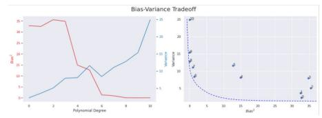
Figure 5.22: Fitting polynomials of increasing degree to the cosine function within the range [-5, 5]. On the left we see that as the degree (complexity) of the model increases, the bias decreases and the variance increases. The plot on the right shows the bias variance tradeoff frontier (dashed line). The frontier has been added to visualize the tradeoff trend, it is not a hard boundary that cannot be crossed.
