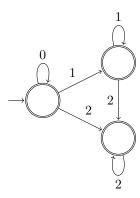
b) The deterministic automaton can be found by applying the power set construction presented in the lecture followed by the state minimization algorithm. However, it is obvious that the automaton shown below does the job.
