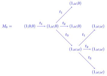
One can merge the equivalent node and obtain the coverability graph:
