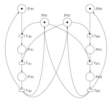
In the following, use  $M = (P_{A0}, P_{A1}, P_{A2}, P_{R1}, P_{R2}, P_{B0}, P_{B1}, P_{B2})$  as marking vector and  $T = (t_{A0}, t_{A1}, t_{A2}, t_{B0}, t_{B1}, t_{B2})$  as firing vector.
