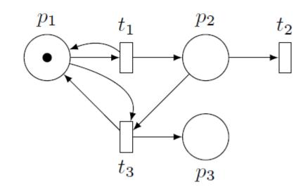
$$M_0 = (1,0,0) \xrightarrow{t_1} (1,\omega,0) \xrightarrow{t_3} (1,\omega,\omega)$$
