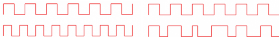
Figure 14.8: Drift (left) and Jitter (right). On top is a square wave, the wall-clock time t^* .
