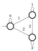
b) The deterministic automaton can be found by applying the power set construction presented in the lecture followed by the state minimization algorithm. However, it is obvious that the automaton shown below does the job.
