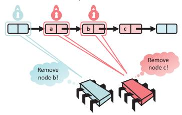
Hand-Over-Hand Locking: Removing Nodes
