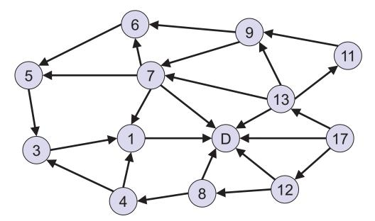
Note that positive labels can be chosen such that higher labels point to lower labels (destination label D = 0).
