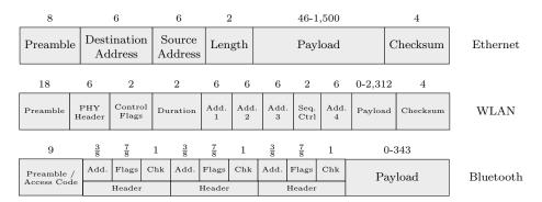
Figure 5.3: The complete physical representations of typical Ethernet, Wireless LAN and Bluetooth packets. The number above each field corresponds to its length in bytes.
