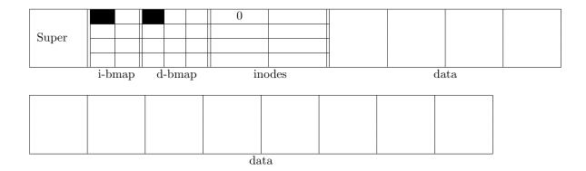
Initially, only inode 0 exists and contains a single pointer to data block 0. This inode represents the root directory. Since the root directory is initially empty, there is no data stored in the data block.
