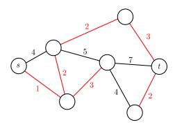
In general, a minimum spanning tree (MST) can be found using Kruskal's algorithm.
