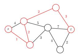
In general, a shortest path can be found using Dijkstra's algorithm.
