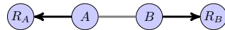
Figure 5.21: The exposed terminal problem: senders A and B could send to their respective recipients R_A and R_B simultaneously, but believe it would cause collisions due to carrier sensing.
