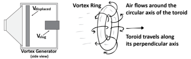
Figure 2: (left) Volume of air moved by speaker equals the volume of the slug used to model the vortex formation. (right) Vortex ring is a toroid where air flows around the circular axis as the entire toroid travels along its perpendicular axis.
